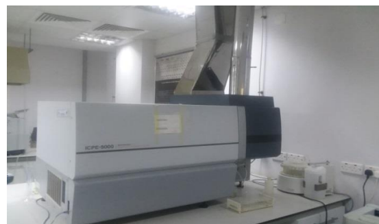
Figure (3) Shimadzu ICPE-9000 Manufactured in Japan
