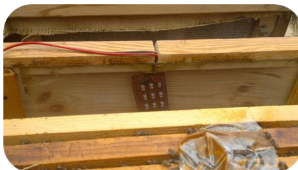
Figure 4. Modified hive with lamps that emit 300-650 nm waves on the inner side of the hive.
